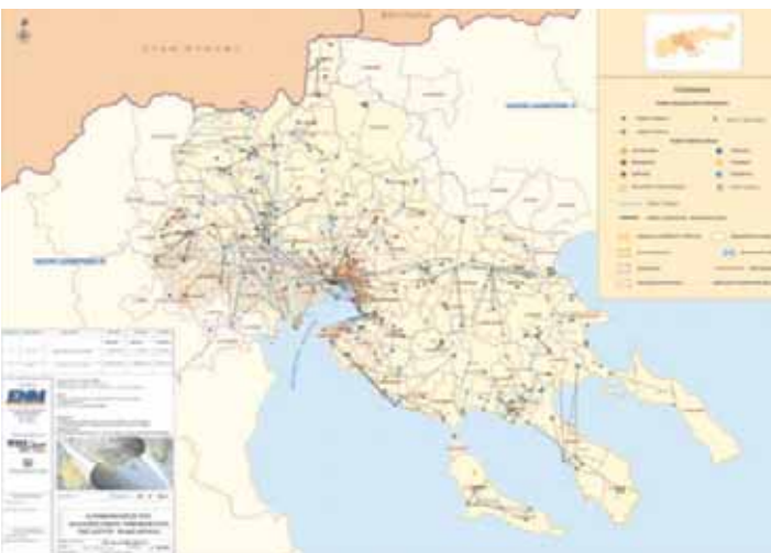
Fig. 7. Example of schematisation of a river network for river basin planning in Greece
